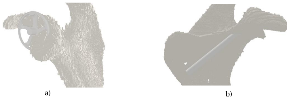
Fig. 3: Static collision configurations used for chunk-size performance testing with: a) reamer and b) peg-hole cylinder tools.
