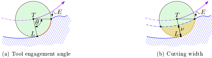
Fig. 1: Illustration of the tool engagement angle \theta and the cutting width \nu at the same point T along the tool path (shown in purple). The green disk depicts the tool. The blue curves stand for the boundary between the area machined and the area not yet machined (that is indicated by the blue hatching).
