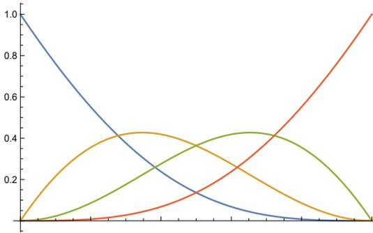
Fig. 1: Basis functions of the up-degreed rational quadratic Bézier curve with  $w = 1/2$ .
