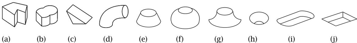
Fig. 2: Applied SFs: (a) Polygonal extrusion, (b) Curved extrusion, (c) Rib, (d) Pipe, (e) Taper, (f) Convex flange, (g) Concave flange, (h) Tapered hole, (i) Curved hole, and (j) Polygonal hole.
