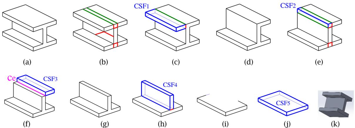
Fig. 4: Example 2: (a) Example 2, (b) ALs and SALs, (c) Detection of CSF1, (d) Extraction of CSF1, (e) Detection of CSF2, (f) Extraction of CSF2 and detection of  $C_e$ , (g) Extraction of CSF3, (h) Detection of CSF4, (i) Extraction of CSF4, (j) Detection of CSF5, and (k) Overview of the solution.
