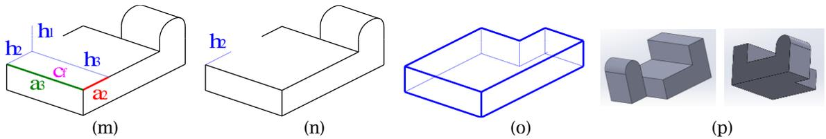
Fig. 3: Example 1: (a) Example 1, (b) Line labeling, (c) Junctions, (d) Additional lines, (e) Detection of two SFs, (f) Curved extrusion with hidden lines, (g) Appeared hidden lines, (h) Extraction of the curved extrusion, (i) Cuboid with hidden lines, (j) Appeared hidden lines, (k) Drawing of an SAL, (l) Detection of another cuboid, (m) Recognition of a contact face, (n) Removal of unnecessary dotted lines, (o) Detection of a polygonal extrusion, and (p) Two overviews of the solution.
