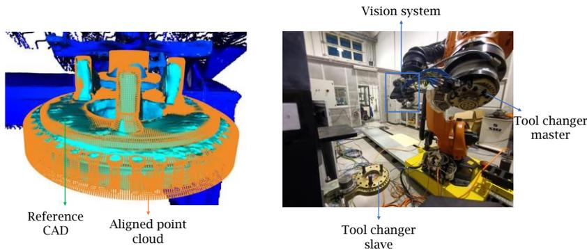
Fig. 4: Left: Alignment of the acquisition result (point cloud in orange) and the reference CAD geometry (green mesh); Right: Final robot configuration with the vision system.
