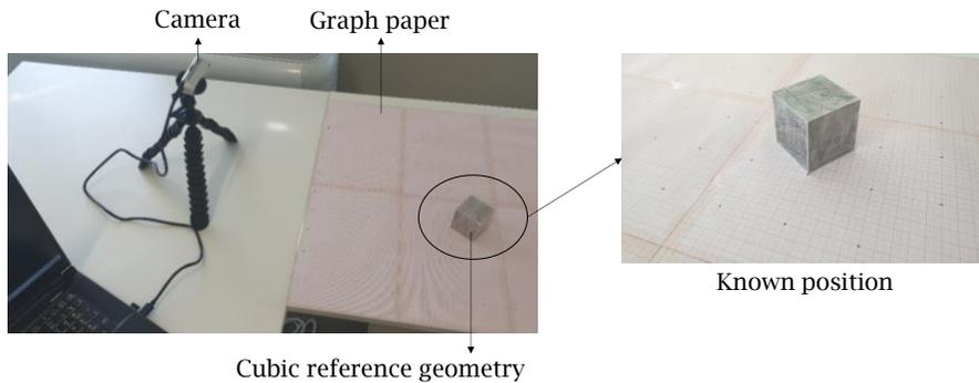
Fig. 2: Testing the ICP algorithm.
