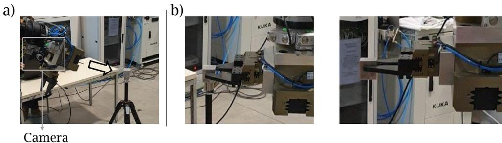
Fig. 3: Pick-and-place operation: a) Detection of the object; b) Pick task.
