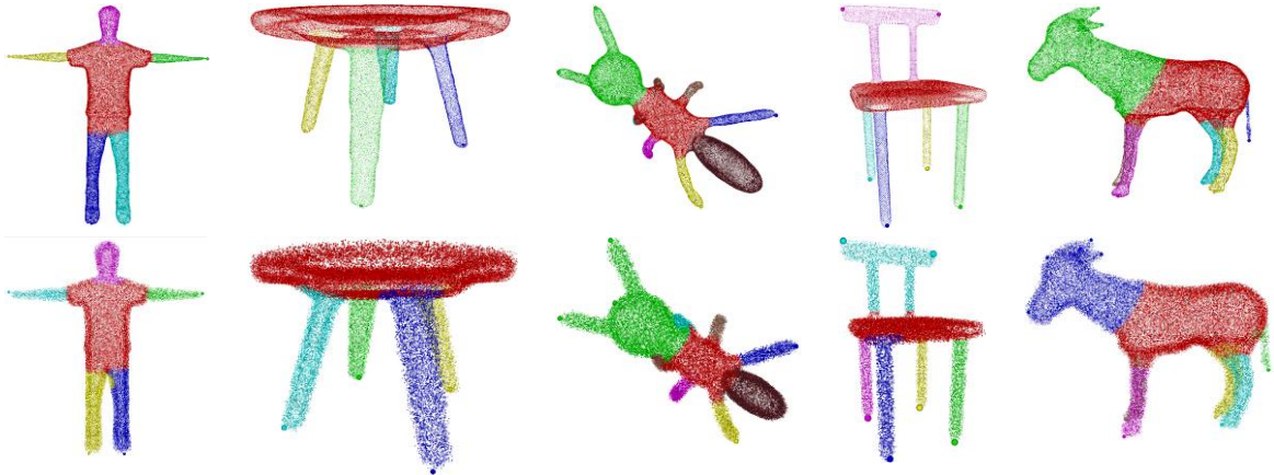
Fig. 2 Semantic segmentation of various point clouds. First row without noise. Second row with noise (1% random displacement of the points from their initial positions).
