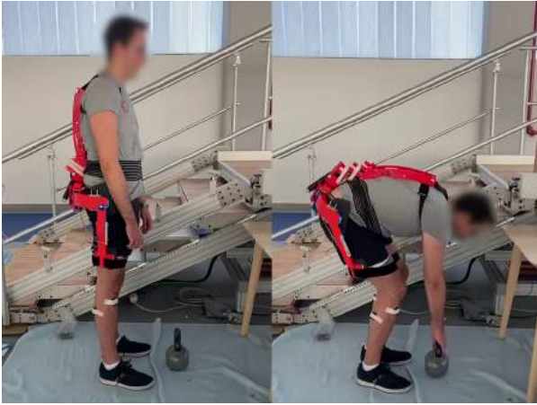
Fig. 1: Operating principle of a low-back exoskeleton based on backbone kinematics.
