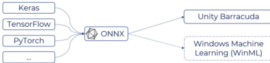
Fig. 3: Communication interface to adapt the model to the mobile support with ONNX.
