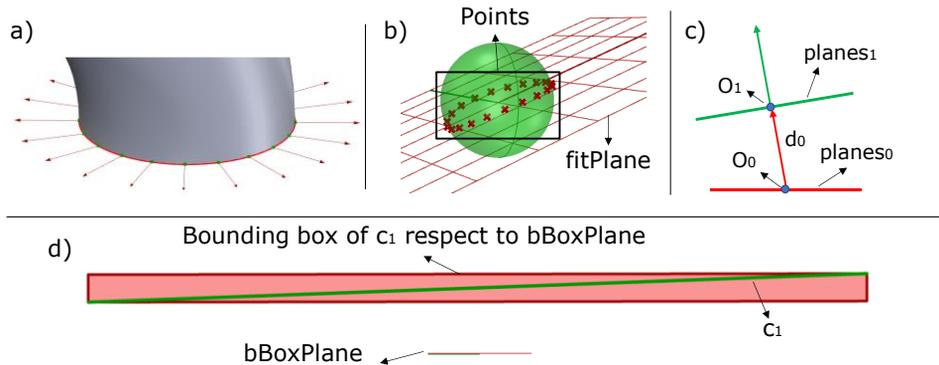
Fig. 3: Non-uniform slicing algorithm: a) Surface normal of the input geometry delimited by  $c_1$  and  $c_n$ ; b) Collection of surface normals in a unit sphere and fitting of a plane; c) Evaluation of the bounding box aligned to the fitting plane.
