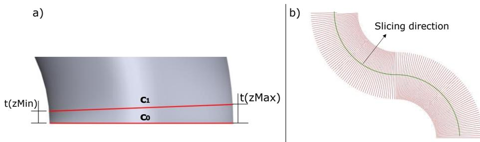
Fig. 4: a) Single non-uniform layer; b) Final result of the slicing process.
