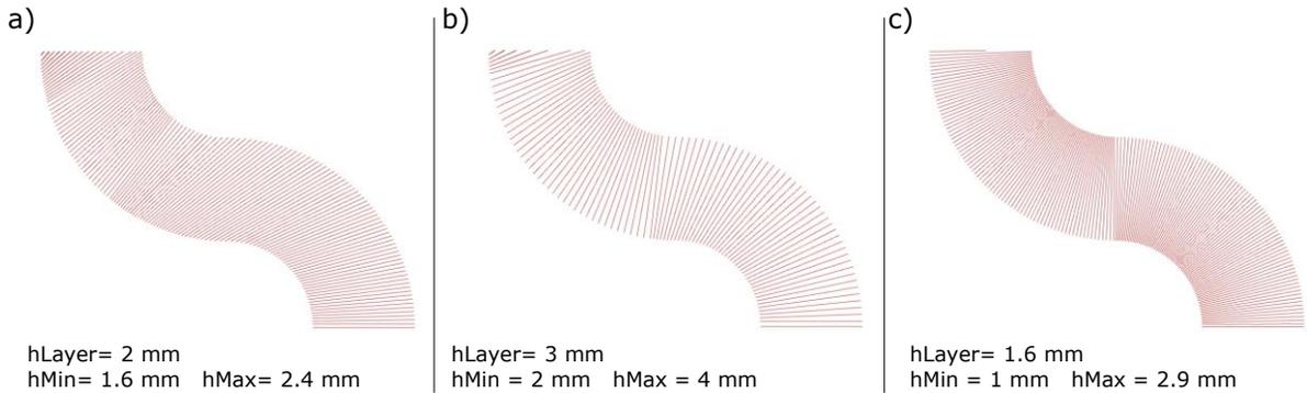
Fig. 6: Non-uniform slicing applied to the same geometry but with different manufacturing limits.
