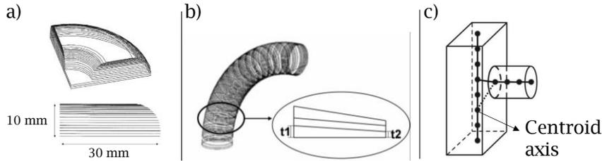
Fig. 1: Reviewed algorithms: a) Adaptive slicing [9]; b) Non-uniform slicing based on minimal enclosing crown algorithm [11], taken from [6]; c) Non-uniform slicing based on centroid axis algorithm [8].
