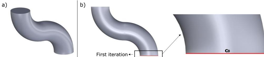
Fig. 2: Non-uniform slicing algorithm: a) Input geometry; b) First iteration of slicing.
