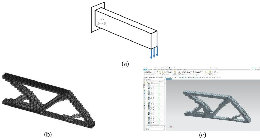
Fig. 4: Topology optimization of a 3D cantilever beam: (a) Design domain and boundary conditions, (b) Matlab plotted optimized result (reproduced), (c) Automatic CAD model construction.
