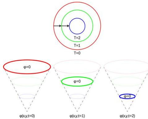
Fig. 1: Level-set function and boundary propagating.
