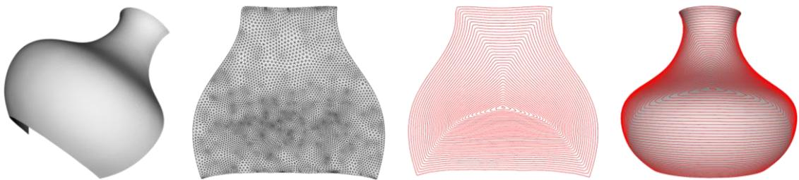
Fig. 2: Toolpath generation for the vase model: (a) 3D mesh surface model, (b) 2D planar mesh, (c) non-uniform offset path on the parametric domain, and (d) iso-scallop toolpath.
