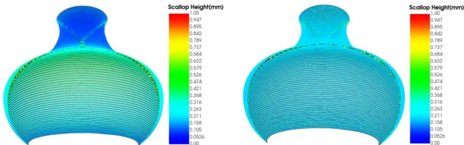
Fig. 3: Scallop height distribution of vase model: (a) uniform offset, (b) non-uniform offset.
