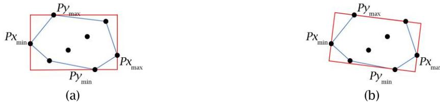
Fig. 4: Build the minimum area bounding rectangle of a convex hull based on the rotating calipers: (a) Build the bounding rectangle, (b) Update the bounding rectangle.
