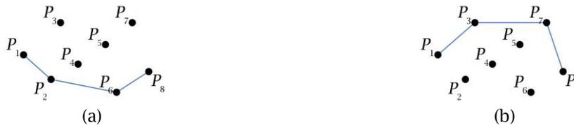
Fig. 3: Compute convex hull based on Andrew algorithm: (a) The lower half of the convex hull, (b) The upper half of the convex hull.
