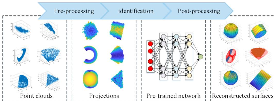
Fig. 1: Overview of the proposed surface reconstruction method based on invariance class identification
