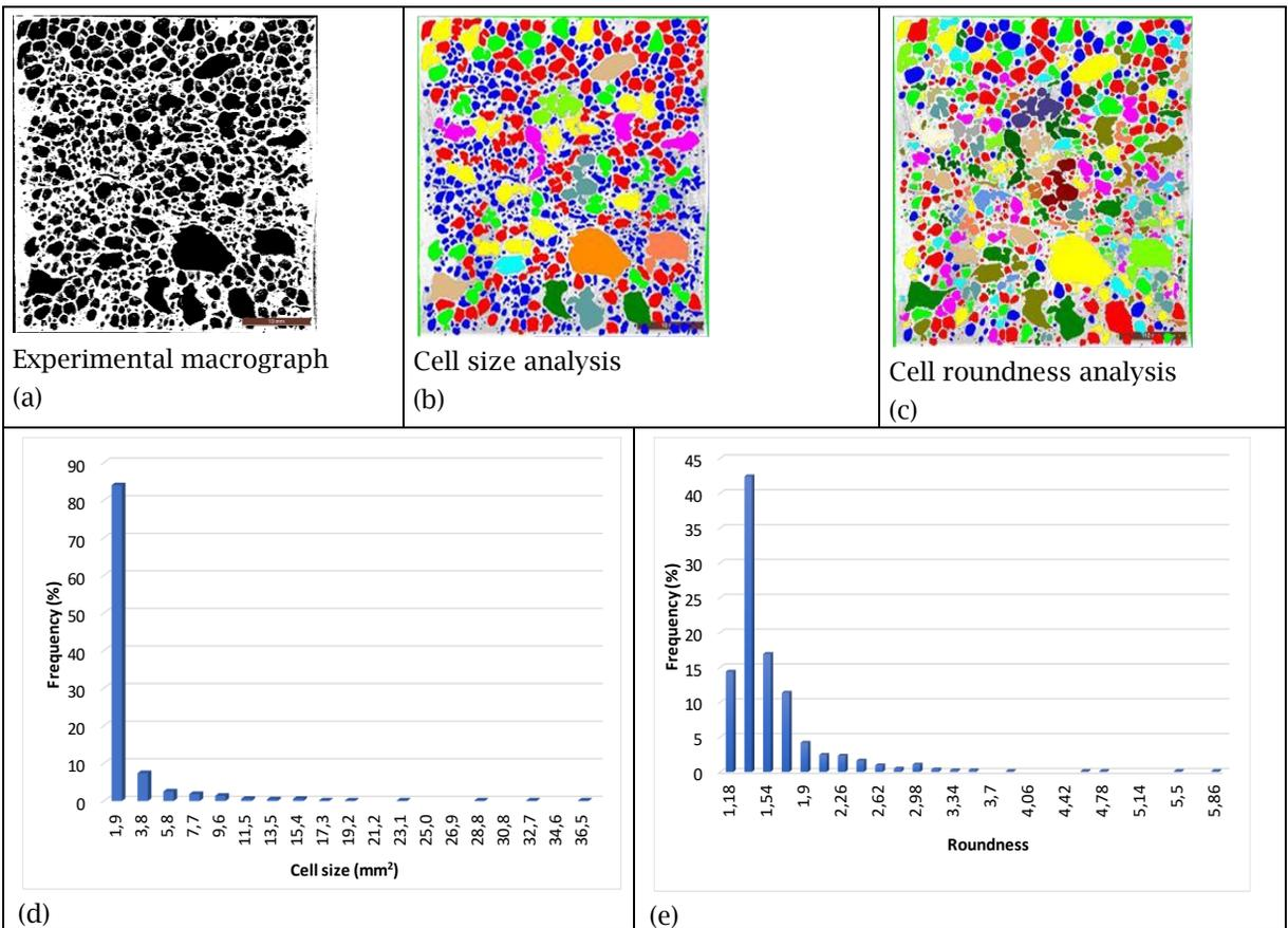
Fig. 1: Foam cell morphology evaluation through transversal cuts.
