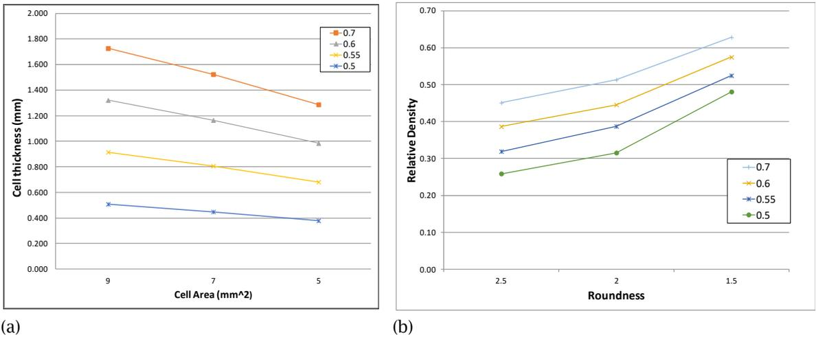
Fig. 3: Sensitivity analysis on final foam geometrical characteristics related to Cell Area and Roundness with different assigned nominal relative densities [0.5;0.7].
