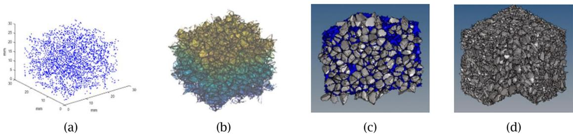
Fig. 2: FEA modeling steps. (a) cell seed; (b) cell convex tessellation; (c) volume definition; (d) FEA solid model.
