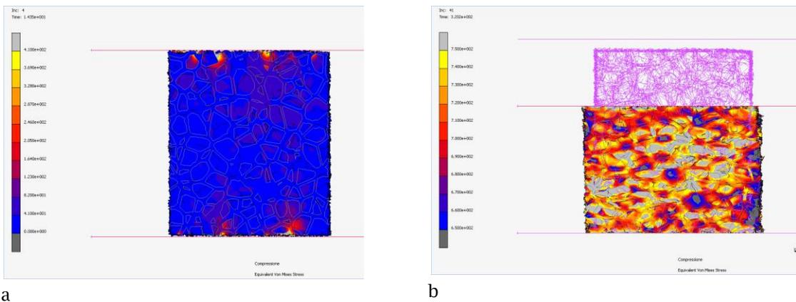
Fig. 4: FEA of the 3D mesoscale model: equivalent Von Mises stress state (MPa) at yielding (a) and at maximum compression load (b).
