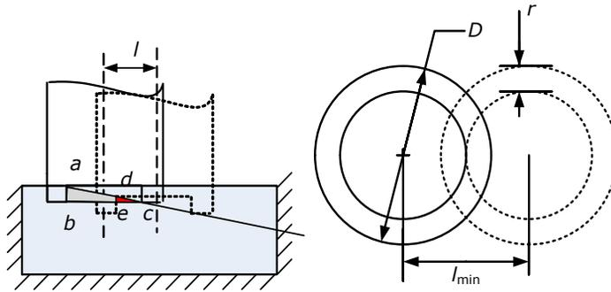
Fig. 2: Selection of ramp length in horizontal direction.
