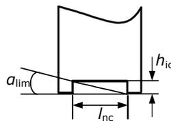
Fig. 3: Critical ramp angle.
