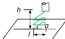
Fig. 1: Schematic diagram of the ramp approach.
