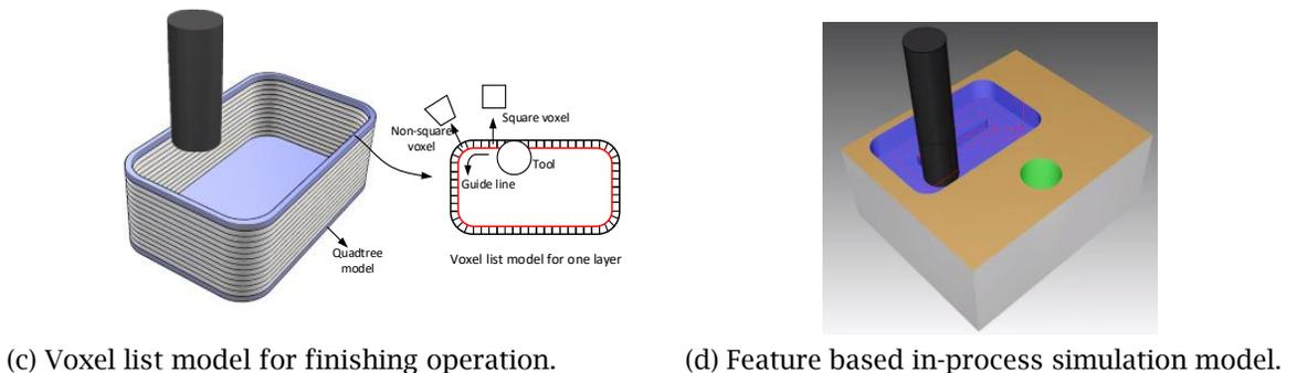
Fig. 1: Illustration of the principles of the customized simulation methods.
