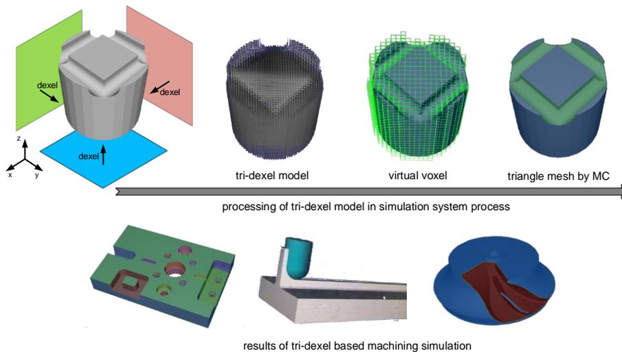
Fig. 2: Tri-dexel model-based machining simulation process.
