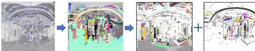
Fig. 3: Extraction of planes and cylinders: (a) Point cloud, (b) Segmentation, and (c) Planar and cylindrical regions.
