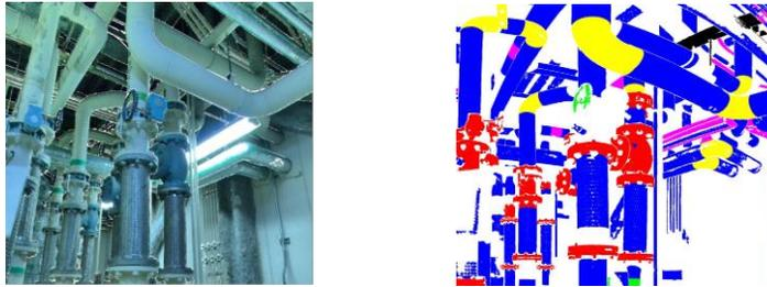
Fig. 8: Classification results: (a) Point cloud, and (b) Classification result.
