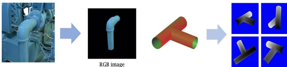
Fig. 6: Generation of images from point clouds: (a) RGB image, and (b) Depth image generated from CAD model.
