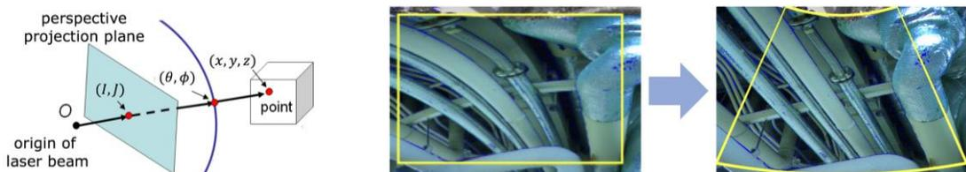
Fig. 5: Generation of images from point clouds: a) Perspective projection, and (b) Conversion to the perspective image.
