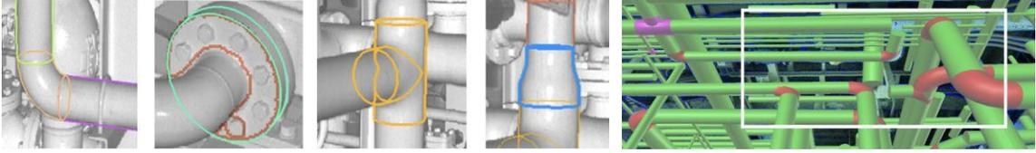
Fig. 1: Component detection using cylinder and plane: (a) Detection of standard parts from cylinders and planes, and (b) Ambiguous pipe routing.
