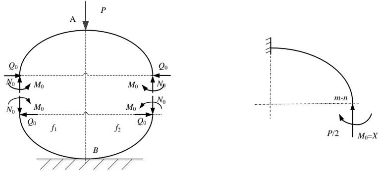
Fig.1: Ring force diagram: (a) Schematic diagram of internal, (b) Quarter ring force diagram.
