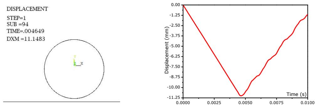
Fig. 3: Process result: (a) Displacement animation capture image, (b) Node displacement change.
