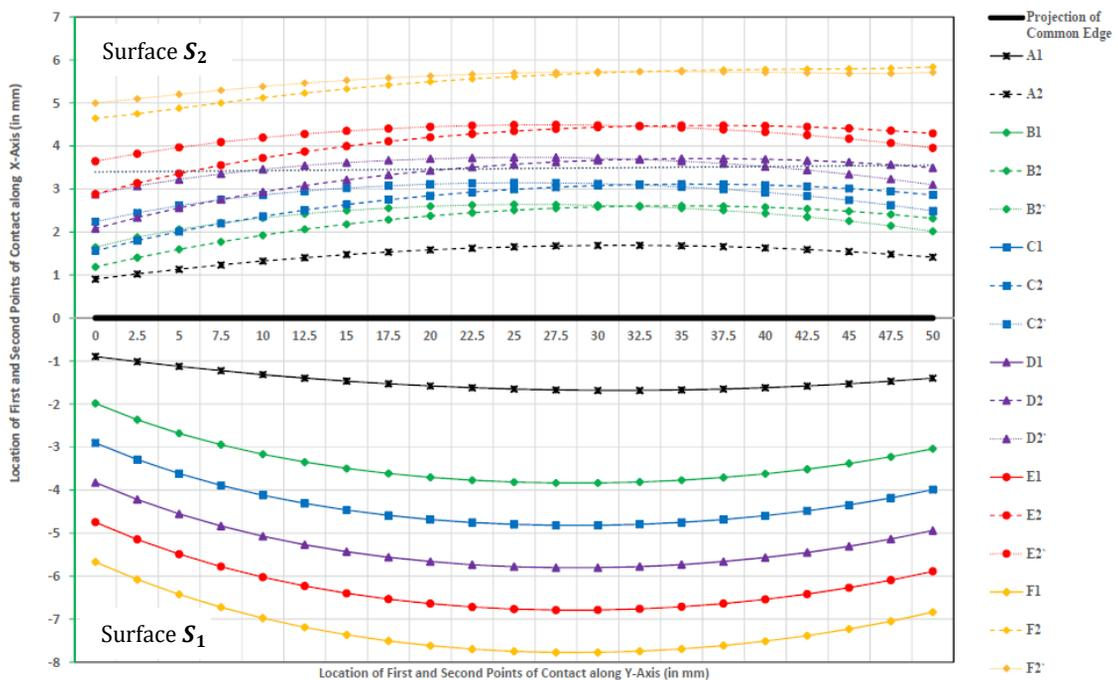
Fig. 4: Trajectories of first and second points of contact for multi-pass finish machining of common edge region between two intersecting Bi-quadratic convex Bezier surfaces. First point of contact on  $S_1$  and second point of contact on  $S_2$ .
