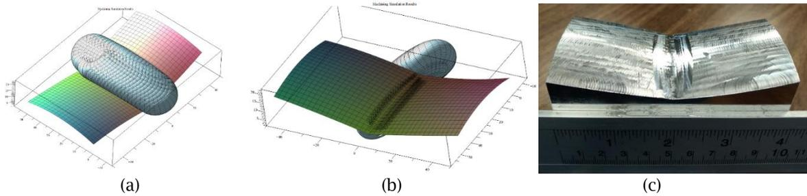
Fig. 5: Simulation of multi-pass tool paths for finish machining of common edge between two intersecting Bi-quadratic convex surfaces: (a) Top view, (b) Bottom view and (c) Machined on DMU-80P-Hi-Dyn tilt-rotary simultaneous 5-axis machining.
