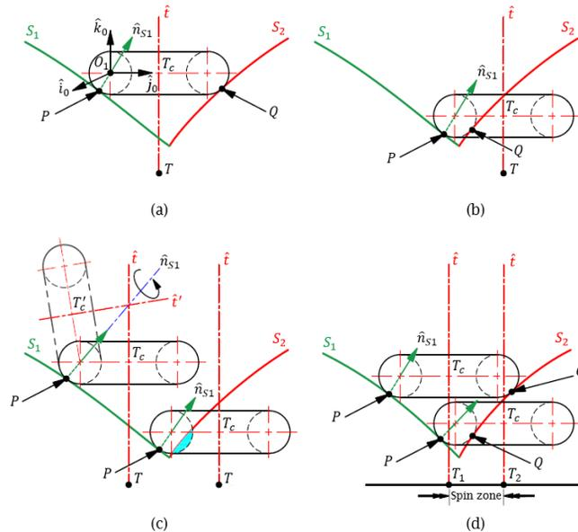
Fig. 3: Determining “Spin Zone” for a given pair of intersecting surfaces: (a) Dropped tool is tangent to both the surfaces, (b) Dropped tool has pseudo insert circle snugly fit between intersecting surfaces, (c) Infeasible footprint locations for DSM method and (d) Definition of limiting toolpath footprint locations for the spin-zone.
