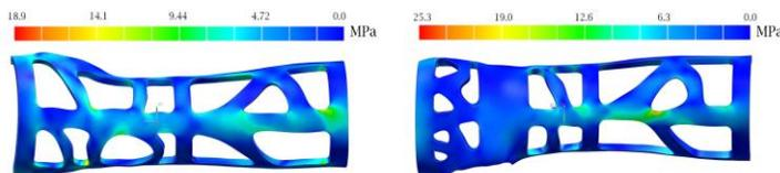
Fig. 2: FE analysis results for the *Small* orthosis, under the *Flexion* load (internal and external surface).
