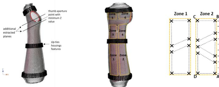
Fig. 3: a) Extraction of the two planes defining the wrist area; b) the six zones of the dorsal pattern; c) template of the holes to be adapted for zone 1 and 2.
