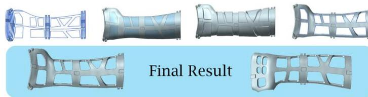
Fig. 4: Phases of the CAD holes adaptation.
