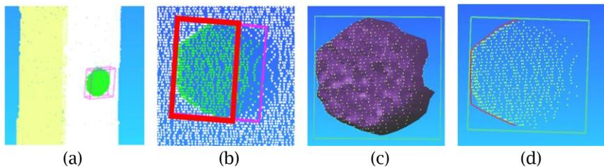
Fig. 5: Process of hexagonal fitting: (a) Cuboid for Bolt Points, (b) Points on the Scanner Side, (c) Triangulation of Bolt Points, and (d) Boundary Points on the Scanner Side.
