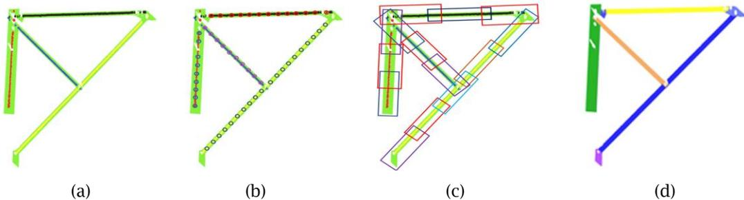
Fig. 3: Process of steel material detection: (a) Center Lines of Planar Regions, (b) Calculation of Residuals of Plane Fitting at Points on the Center Lines, (c) Small Regions along the Center Lines, and (d) Detected Planar Regions.
