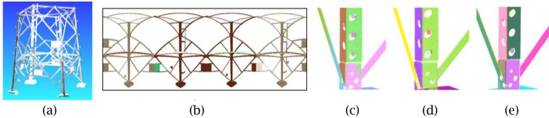
Fig. 2: Extraction of steel materials: (a) Point-Cloud, (b) Segmentation on 2D Lattice, (c) Initial Planes, (d) Merged Planes, and (e) Detected Planes of Steel Materials.
