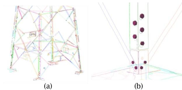
Fig. 8: Detection of steel materials and bolts: (a) Detected Steel Materials and Bolts, and (b) the Close-Up.
