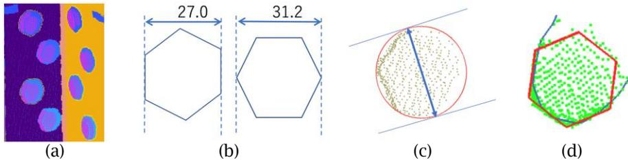
Fig. 4: Two methods for estimating the bolt size: (a) Bolt Points, (b) The Minimum and Maximum Lengths of Bolt, (c) Bolt Size Estimated by the Maximum Width Method, and (d) Bolt Size by the Hexagonal Fitting Method.
