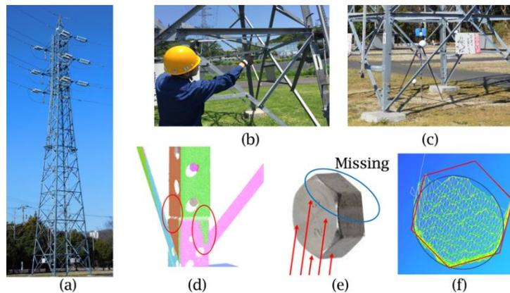
Fig. 1: Measurement of pylons: (a) Steel Tower, (b) Manual Measurement, (c) Laser Scanning on the Ground, (d) Detection of Planes of Steel Materials, (e) Laser Scanning of Bolt, and (f) Point-Cloud of Bolt.
