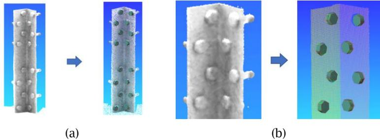
Fig. 6: Detected bolts from a point-cloud: (a) Detected Bolts, and (b) the Close-Up.
