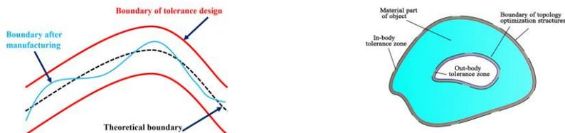
Fig. 2: (a) Boundary of tolerance simulation models, (b) Two types of tolerance zones.
