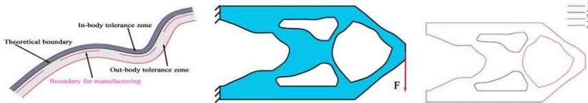
Fig. 3: (a) Asymmetric tolerance zone and machining boundaries, (b) Topology optimization structure, (c) Contour segmentation for tolerance analysis.
