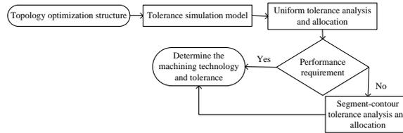
Fig. 1: Tolerance design of the topology optimization structure.
