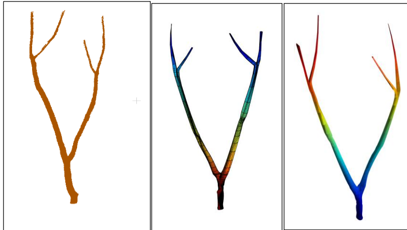
Fig. 4: Point Cloud Data and Resulting Multi Branch Surface Model.
