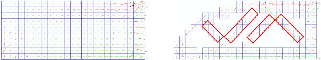
Fig. 2: Stress fields: (a) in original structure, (b) in optimized structure.
