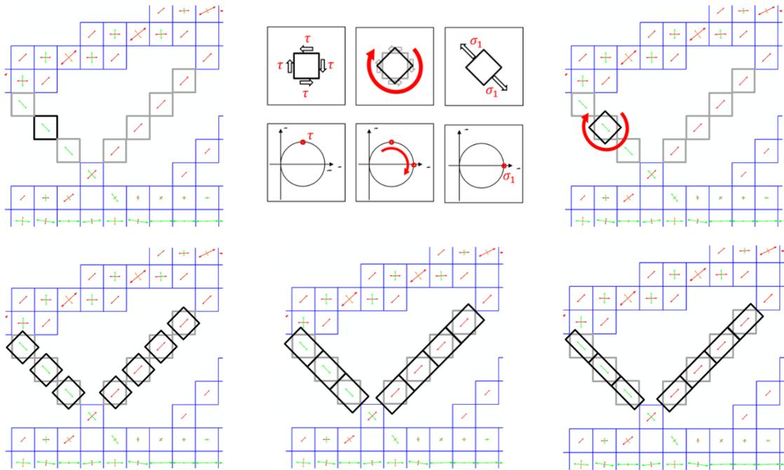
Fig. 3: The re-mesh procedure: (a) stress tensor of the elements, (b) calculation of the angle between original and principal reference system using the Mohr circle, (c) rotation of a single element, (d) rotation of many adjacent elements, (e) connection of separated adjacent elements, (f) size optimization of connected elements.
