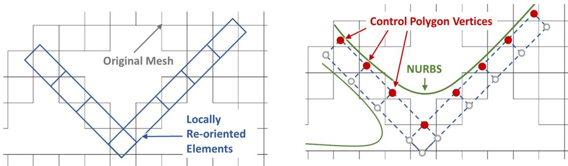
Fig. 4: NURBS application: (a) re-oriented elements, (b) definition of fitting NURBS.
