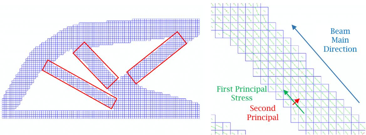
Fig. 1: Result of the process of topological optimization using a sensitivity filter: (a) the whole resulting topology, (b) a particular of a sub-structure, and principal stress tensor.
