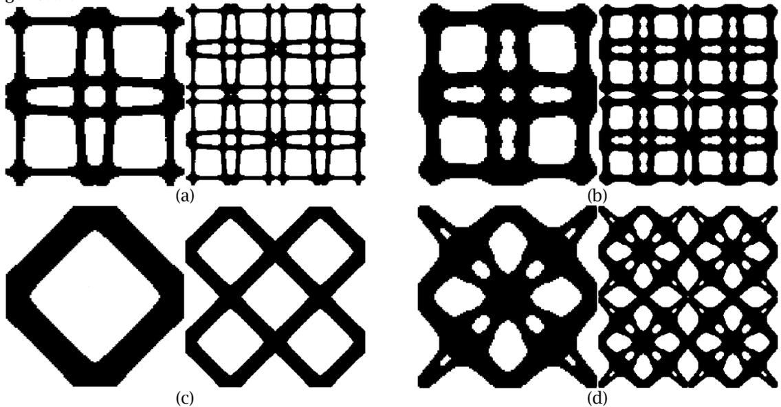
Fig. 1: Examples of the meta-material topology optimization, (a)  $\bar{E}_{11} = \bar{E}_{22} = 0.3$  and  $V_{max} = 0.4$ , the single- and 2\*2 multi-unit views, (b)  $\bar{E}_{11} = \bar{E}_{22} = 0.5$  and  $V_{max} = 0.6$ , the single- and 2\*2 multi-unit views, (c)  $\bar{E}_{33} = 0.14$  and  $V_{max} = 0.4$ , the single- and 2\*2 multi-unit views (d)  $\bar{E}_{33} = 0.2$  and  $V_{max} = 0.6$ , the single- and 2\*2 multi-unit views
