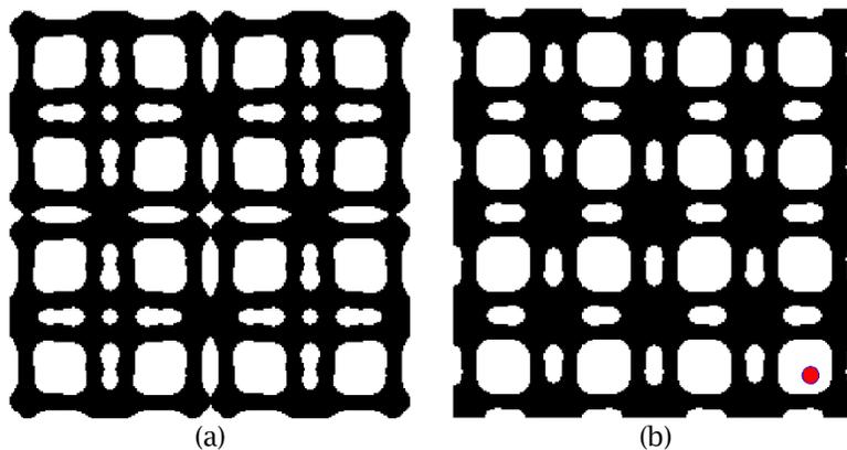
Fig. 3: A comparative case study, (a) result from Fig. 1b without curvature control, (b) result with curvature control (the red dot indicates lower limit of the radius of the curvature).
