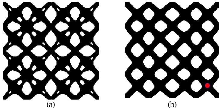
Fig. 2: A comparative case study, (a) result from Fig. 1d without length scale control, (b) result with component length scale control (the red dot indicates lower limit of the component length scale)
