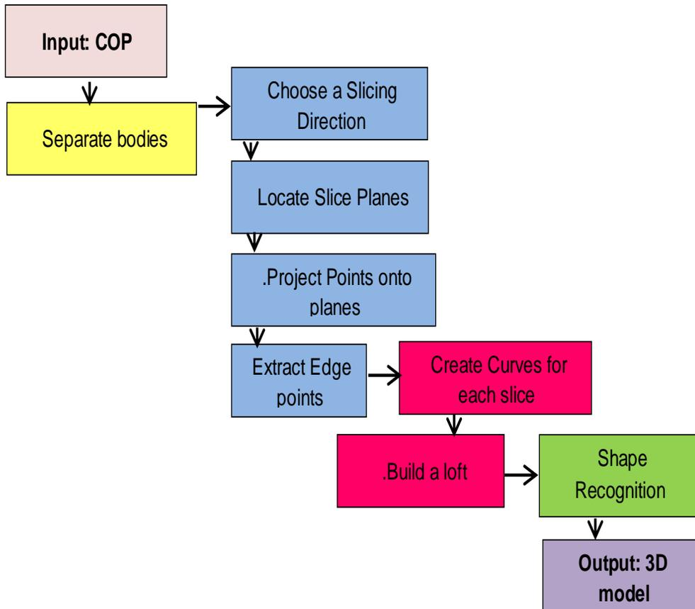
Fig. 2: Block Diagram of the solution process.
