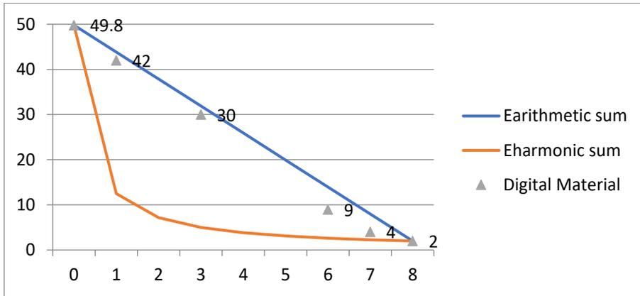
Fig. 6: The tensile strength relationship between the digital material and the proposed material limits.
