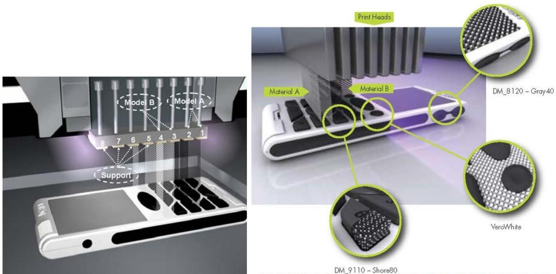
Fig. 1: The PolyJet Matrix printing block and its working principle [10].
