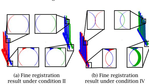
Fig. 6: Fine registration results of non-overlapped point clouds.
