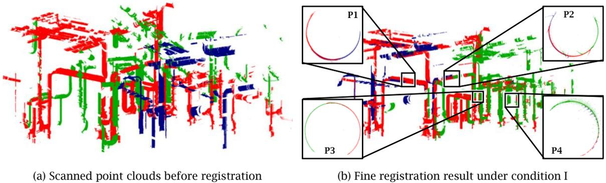
Fig. 7: Results of coarse and fine registration for an HVAC plant under conditions I.
