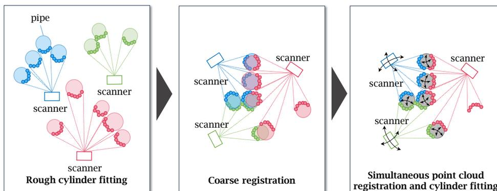
Fig. 1: Registration and model fitting of scanned points of piping systems.
