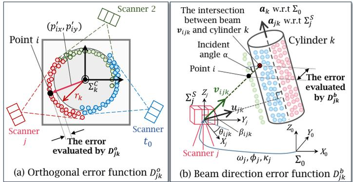
Fig. 3: (a) Orthogonal error function and (b) beam direction error function.
