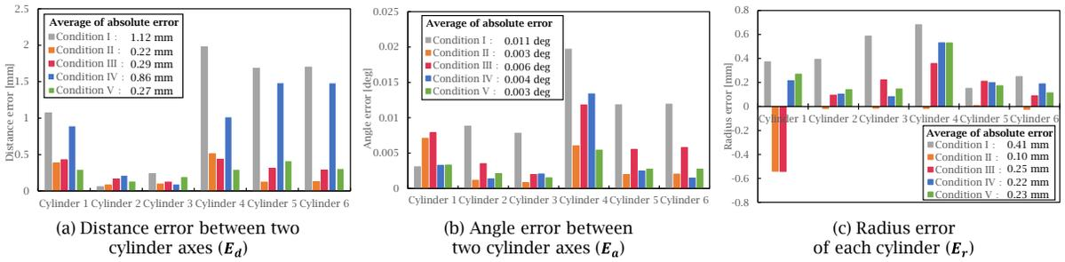
Fig. 5: Error distributions after fine registration under conditions I to V.
