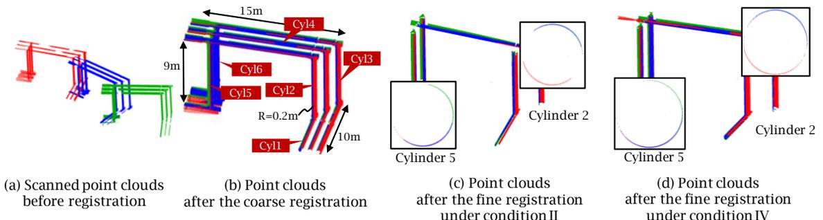
Fig. 4: Results of coarse and fine registration under conditions II and IV.
