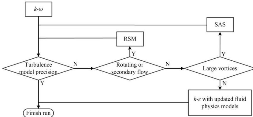
Fig. 3: Subroutine for advanced turbulence models.
