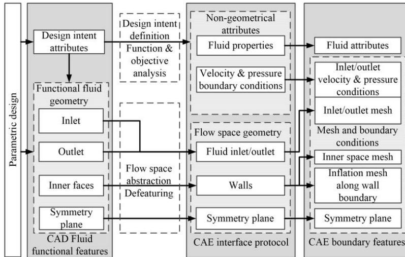
Fig. 1: Feature conversion between the design view and the analysis view.
