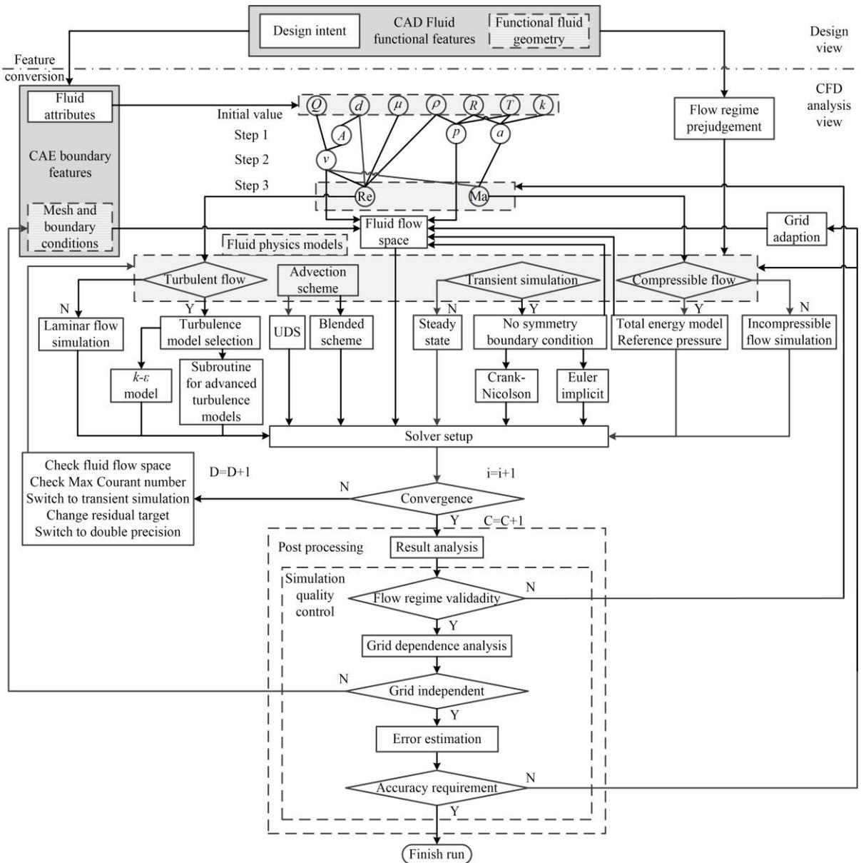
Fig. 2: Intelligent solver functions for the dry steam simulation.
