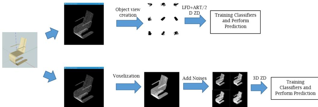
Fig. 2: The classification procedure applied to a chair model.
