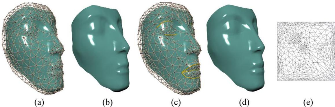
Fig. 1: Degree 3 D1RC-spline surfaces. (a) Input triangular mesh; (b) The D1RC-spline surface; (c) Specify sharp edges (in yellow) on the control mesh; (d) The resulting D1RC-spline surface with sharp features; (e) The parameterization of the input mesh in (a).
