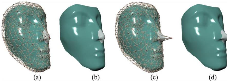
Fig. 3: The influence region of a control point in a degree 3 D1RC-spline surface. (a) The D1RC-spline surface and the control mesh, where the selected control point and his influence region are visualized in red and white, respectively; (b) The D1RC-spline surface; (c) The selected control point is moved and the shape of the surface is locally adjusted; (d) the adjusted surface.
