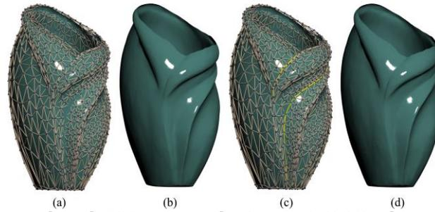
Fig. 5: (a) Input triangular mesh with 820 vertices; (b) Degree 3 D1RC-spline surface; (c) Some edges are labelled as a sharp edges (in yellow); (d) The resulting surface with  $C^0$  continuity along the feature lines corresponding to the labelled edges.
