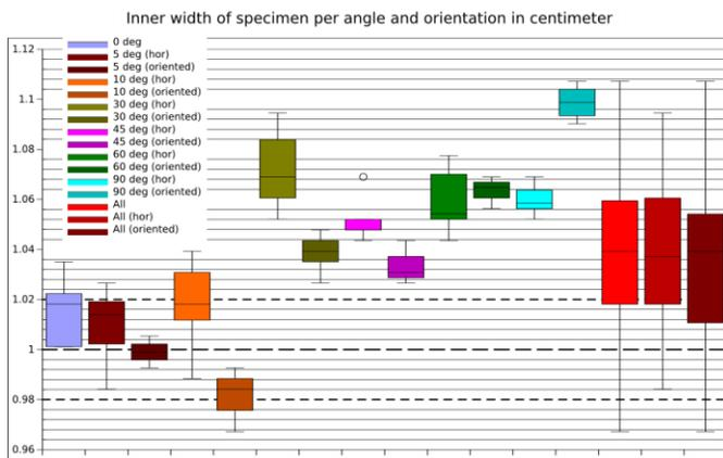
Fig. 5: Inner width of specimen per angle and orientation in centimeter
