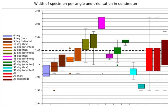
Fig. 3: Width of specimen per angle and orientation in centimeter.
