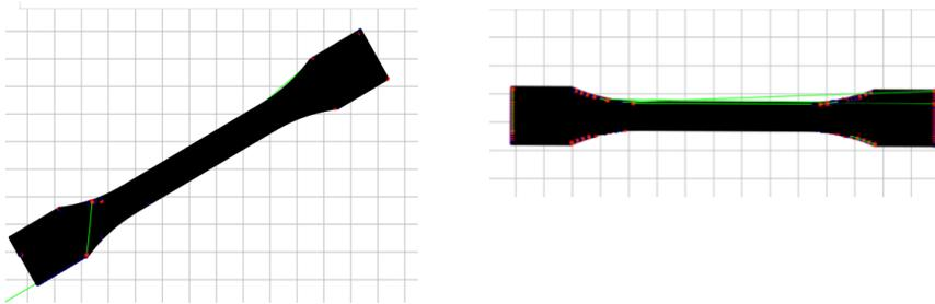
Fig. 1: View of toolpath for object from Test set A (horizontally aligned) on the left (a) and object from Test set B (aligned at angle to X-axis) on the right (b)
