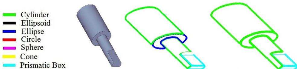
Fig. 3: Here is a sample result from the Engineering Shape Benchmark (ESB) database. : (a) Color Code to interpret results, (b) Input Image, (c) Result without face fusion, and (d) Result with face fusion.
