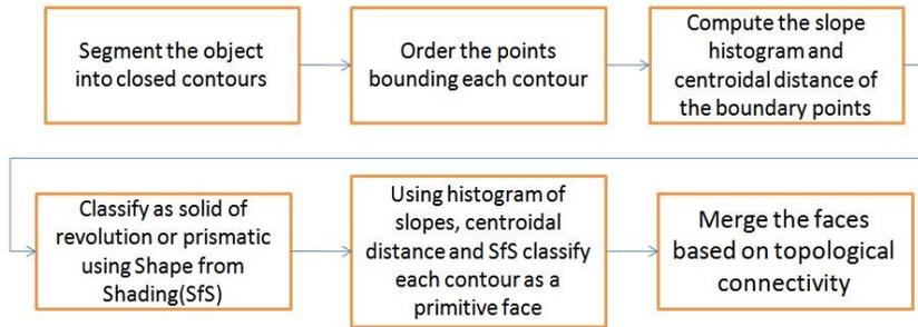
Fig. 2: Overview of the approach to detect primitives.
