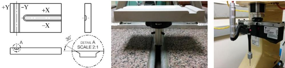
Fig. 1: Calibration target and Renishaw® AM1 adjustment module: (a) Drawing of target, (b) Target and adjustment module, (c) Sensor and adjustment module.
