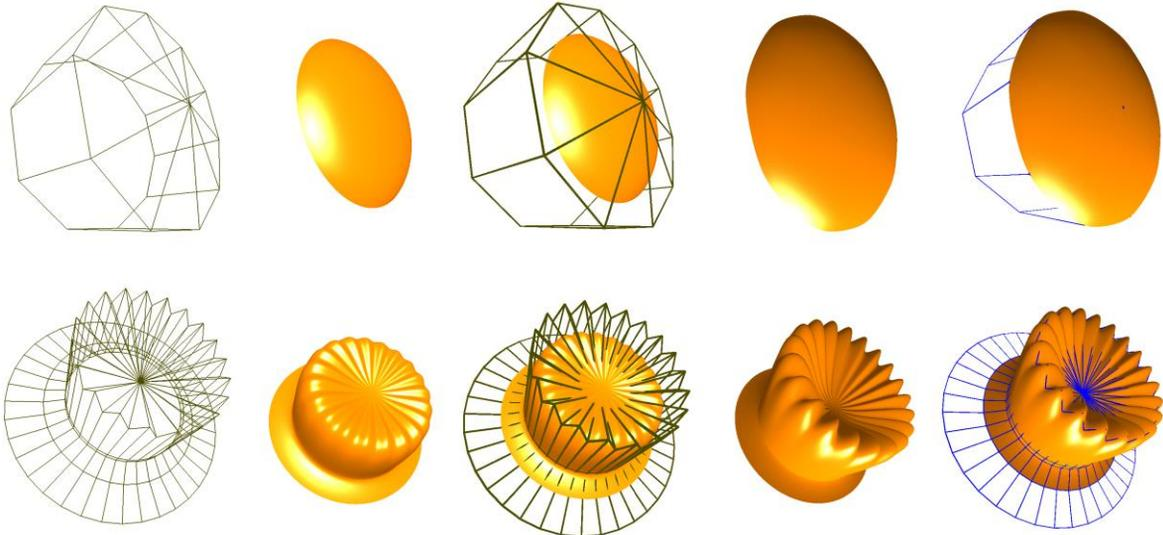
Fig. 4: two examples of interpolation on Polar mesh, (a) mesh, (b) Polar limit surface, (c) mesh with limit surface together, approximating, (d) interpolation surfaces (e) mesh shown with interpolation.
