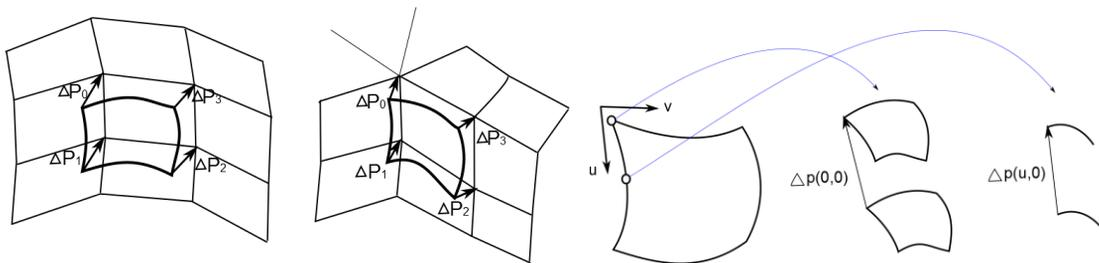
Figure 2: (a) & (b) difference vectors between control points and corresponding CCS limit points, (c), (d) & (e) How can CCS surface and an offsetting surface be added to form an interpolation surface. Bottom of (d) & (e): faces and curves of CCS limit surface; top of (d) & (e) the interpolating surface by adding an offsetting surface of bi-degree 5 Bezier crust working on the given difference vectors.
