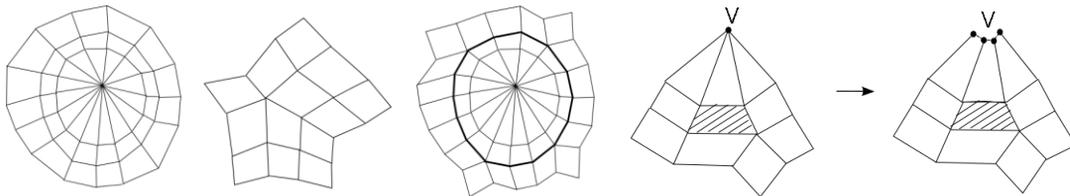
Fig. 1: (a) Polar mesh, (b) Catmull-Clark mesh, (c) Polar Catmull-Clark mesh, (d)-(e) mesh conversion of triangular faces into quad faces at Polar extraordinary points
