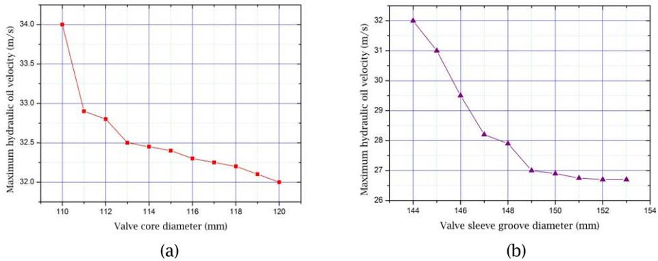
Fig. 6: Maximum velocity: (a) with different valve core diameter, and (b) with different valve sleeve groove diameter.
