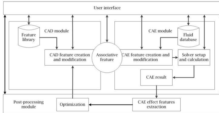
Fig. 4: Prospective CAD/CAE integration system framework.
