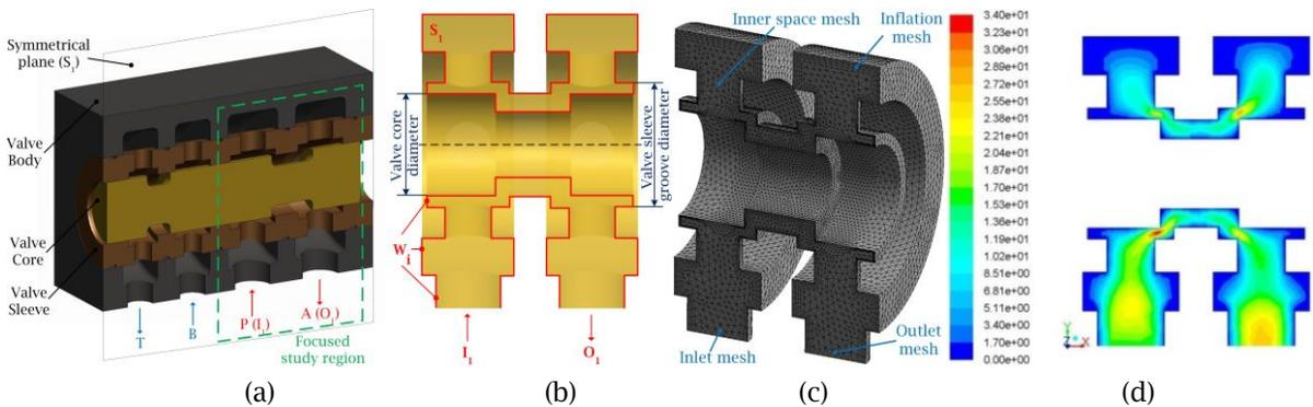
Fig. 5: Case study of a hydraulic valve: (a) Valve structure, (b) Fluid space abstraction (Sectional view), (c) Mesh generation, and (d) Velocity distribution.
