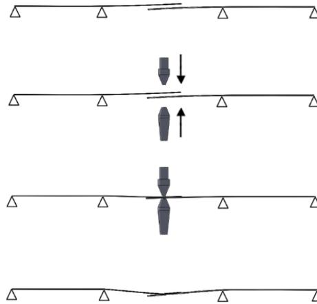
Fig. 2: Assembly process of compliant sheet metal parts [4].
