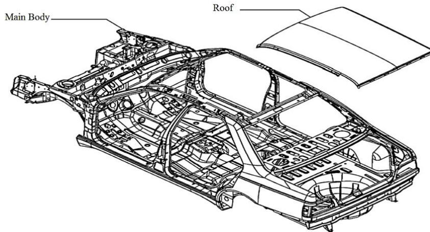
Fig. 1: Main car body components and roof before assembly, courtesy of IKKCO.
