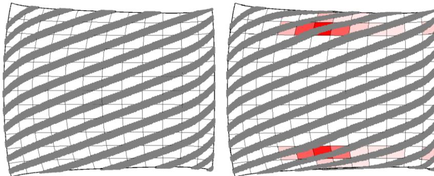
Fig. 4: Highlight bands of nominal (left) and deformed (right) roof.
