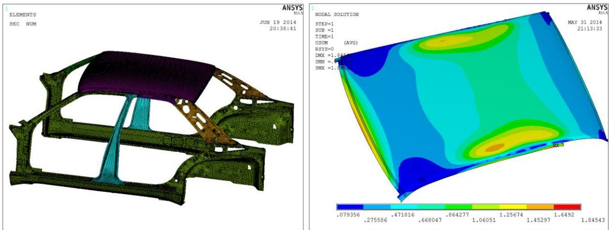
Fig. 3: (a) Example assembly of car body in ANSYS environment (b) Roof’s deformation contour as a result of side bodies’ deviation.
