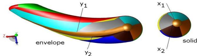
Fig. 2: The envelope of a saucer being swept along a helical trajectory with compounded rotation.
