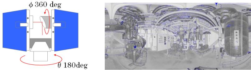
Fig. 1: Depth image defined by two rotating angles.
