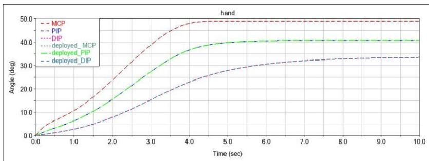
Fig. 6: Rotation angle of finger with and without deployment mechanism.
