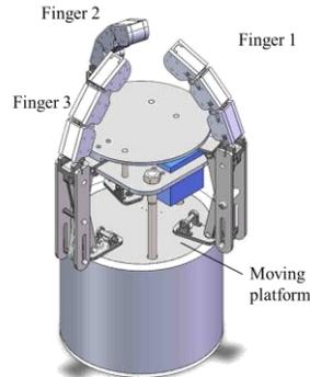
Fig. 1: Overall structure of the robotic hand.
