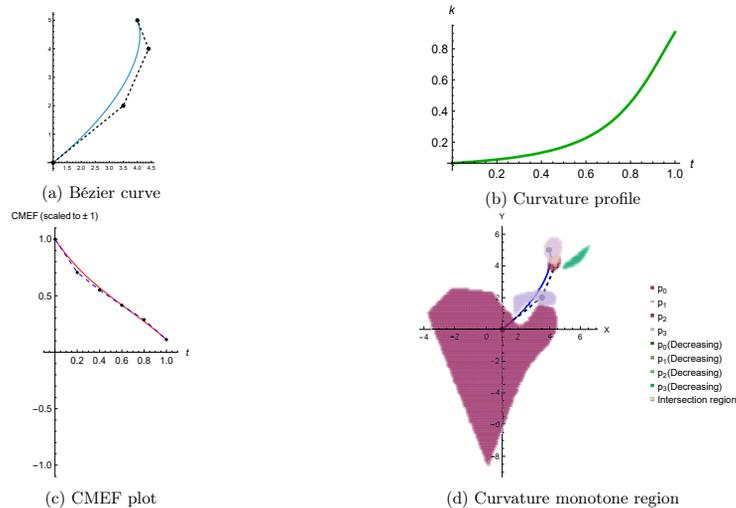
Fig. 1: Example of monotone curvature increasing.
