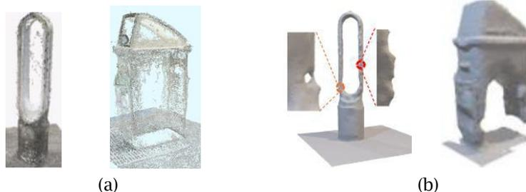
Fig. 1: Point clouds acquired by a mobile device and generated 3D meshes [3]: (a) Low-quality point clouds and (b) Meshes generated by existing methods.
