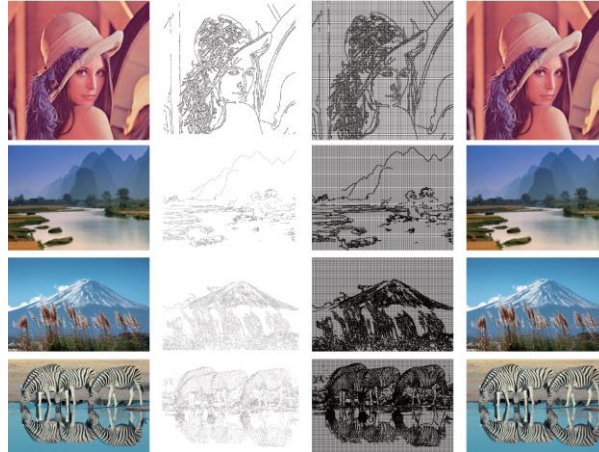
Fig. 5: Fitting high resolution image data. From left to right: raw image, feature extraction results, T-mesh, fitting image.
