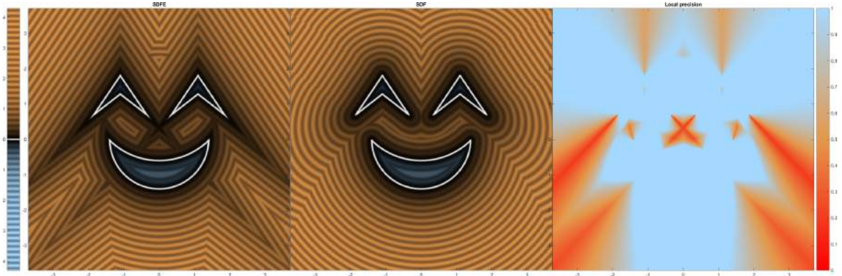
Fig. 2: Left: SDFE obtained through min and max set operations using transformations of a half-plane (line) and a circle primitive. The ratio of the SDFE (left) and the exact SDF (middle) is displayed on the right. The right image shows that the precision of the final SDFE is around 0.2 at maximum. We prove that there is a lower bound to the precision and thus a maximum slowdown for sphere tracing.
