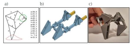
Fig. 1: The design activity, a Jansen's leg structure a) structure and motion profile b) CAD model and c) printed prototype. Image from [1].
