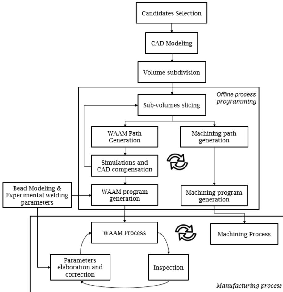
Fig. 1: General framework to approach a WAAM hybrid manufacturing process.
