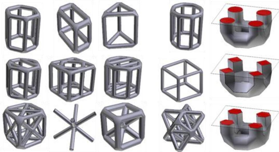
Fig. 2: 3D models of 12 typical lattice unit cells. The right-most column shows three typical cross-section shapes of lattice bars.
