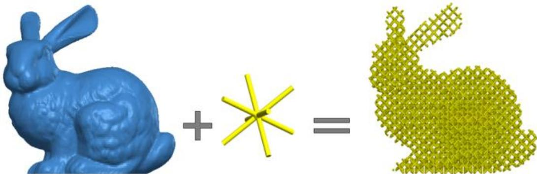
Fig. 4: A model of rabbit filled by lattice structure frame.
