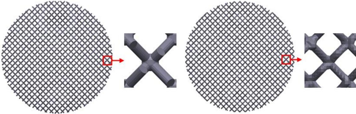
Fig. 5: Modeling result comparison between proposed method (left) and NX software (right).
