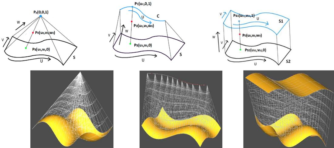
Fig. 6: Enclosed space and corresponding frame models, from left to right: (a) point-to-surface, (b) curve-to-surface, (c) surface-to-surface.
