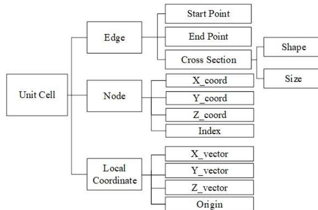
Fig. 1: Universal data structure for describing lattice structures.
