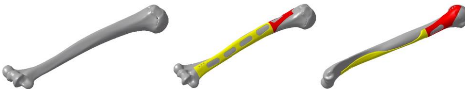
Fig. 3: Left: CAD-model of the humerus CT-scan. Middle and right: Different CAD-model views of the humerus with a customized implant for 3D printing.
