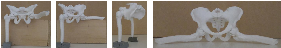
Fig. 10: 3D prototype: (a) Abduction movement of the femur at 90°; (b) Flexion movement of the femur at 90°; (c) Anteversion movement of the pelvis at 90° and (d) Abduction movement of the femur at 70°.
