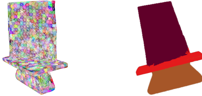
Fig. 2: Left: The first output is the super-voxel obtained by the local point cloud through local iterative clustering, and each super-voxel is marked with colour point cloud block.; Right: The second output is the result of Constrained Planar Cuts based on the concavity and convexity, that is, the various parts of the blade, such as blade body, platform and tenon, are marked with different colours.
